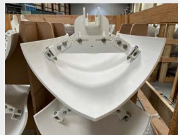
Manufacturing and assembly of double curved parts of the façade.
